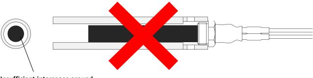
Insufficient interspace around heating element
