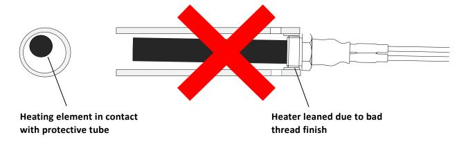
Please make sure to let an interspace of minimum 3mm around the ceramic heating element and the tube.
