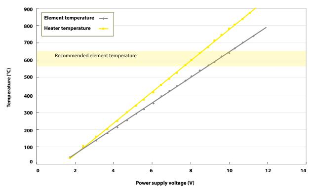
Measured temperature at 20°C. Heater temperature maximum change rate 180°C/s.
