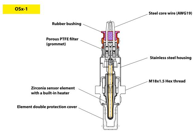
The advanced design of DENSO Lambda Sensors eliminates oxidation and corrosion problem. The unique aluminum oxide double trap layer surrounding the sensor's ceramic element protects it from problem of fuel and maintaining its lifespan and efficient performance.
